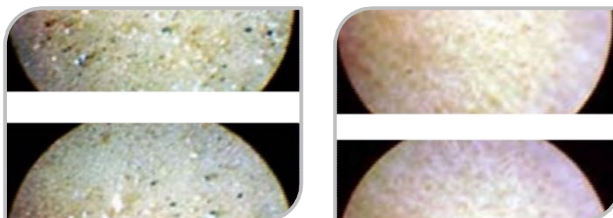
Before cleaning 13 - 17 class according to GOST 17216 After cleaning, 2 - 4 class according to GOST 17216
