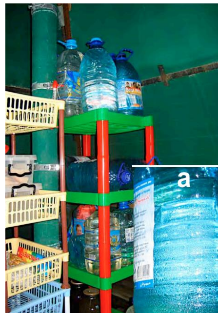
Fig. 4. Inside the pyramid; dew condensation on the outer surface of bottles with water at an ambient temperature of 35 °C
